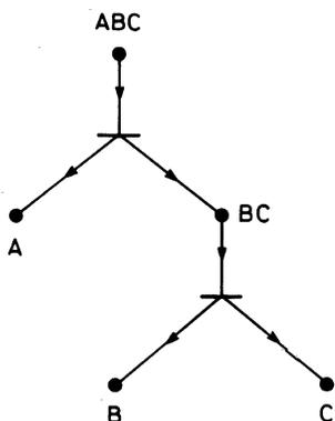
Fig. 8. P-graph representation of a process structure involving sharp separation of mixture *ABC* into its three components.
