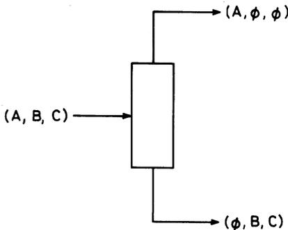
Fig. 3. Operating unit separating mixture  $ABC$  into component  $A$  and mixture  $BC$ .
