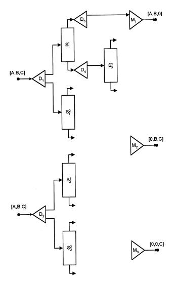
Fig. 21. Creating separator  $S_3^2$  and linking it to the outlet of divider  $D_4$ .
