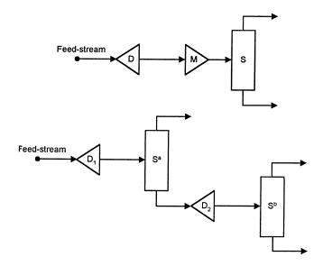
Fig. 13. Examples of a sample and a non-simple path. (a) Simple path: from Feed-stream to S. (b) Non-simple path: from feed-stream to  $S^{b}$ .
