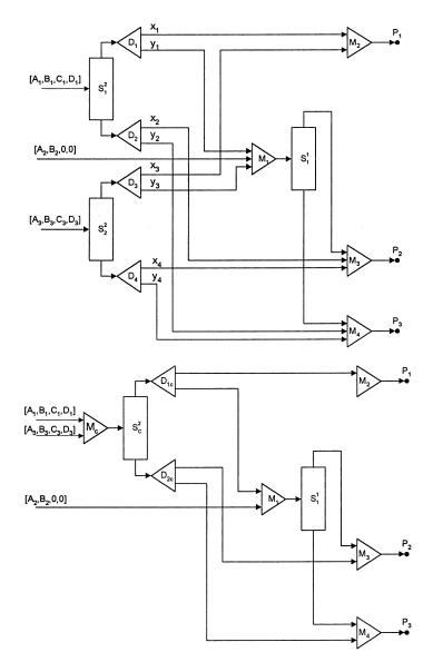
Fig. 4. Illustration of merging separators. (a) Network prior to merging separators identical in type and with the same cost function. (b) Network resulting from merging the separators as indicated in (a).
