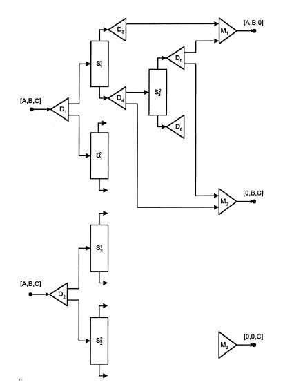
Fig. 24. Establishing two bypasses from the outlet of divider  $D_5$ , one to mixer  $M_1$  for product-stream [A, B, 0] and the other to mixer  $M_2$  for product-stream [0, B, C].
