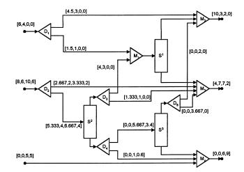
Fig. 10. Optimal structure for Example 2 with combined separators (cost = 104.26).
