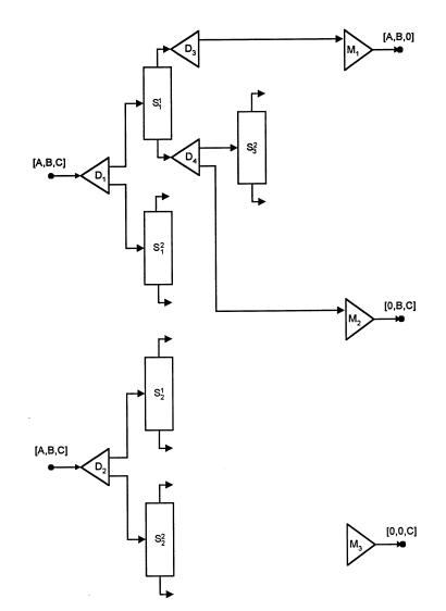
Fig. 22. Establishing a bypass from the outlet of divider  $D_4$  to the inlet of mixer  $M_2$  for product-stream [0, B, C].
