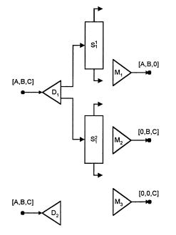
Fig. 17. Creating separators  $S_1^1$  and  $S_1^2$  and linking both of them to the outlet of divider  $D_1$ .
