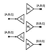
Fig. 16. Creating and linking a divider to each feed-stream and a mixer to each product-stream.
