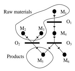
Figure 2. PNS network involving three operating units and six materials
