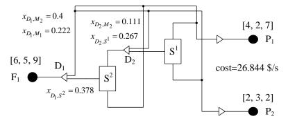
Figure 6. Solution structure of the example with SNS notation
