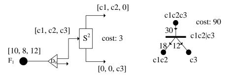
Figure 3. Representation of a separator and the corresponding operating unit
