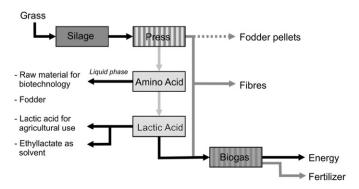
Fig. 2. Flow sheet of a "Green Bio-refinery", Wachter et al. [3].
